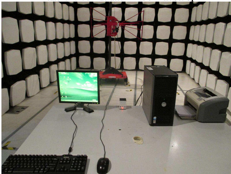
Measurement of Radiated Emission Test Set Up
