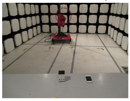
Measurement of Radiated Emission Test Set Up
