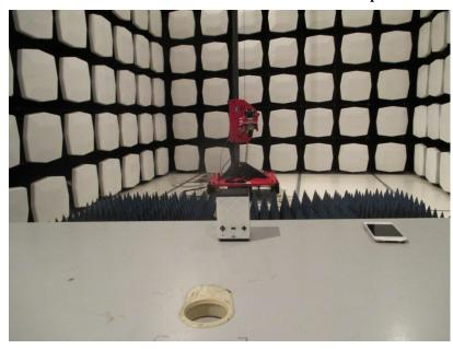
**Measurement of Conducted Emission Test Set Up**
