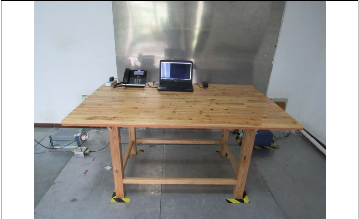
Conducted Emissions Setup Front View
