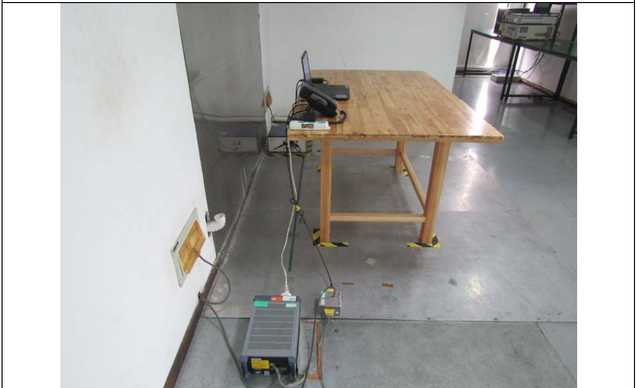
Conducted Emissions Setup Side View
