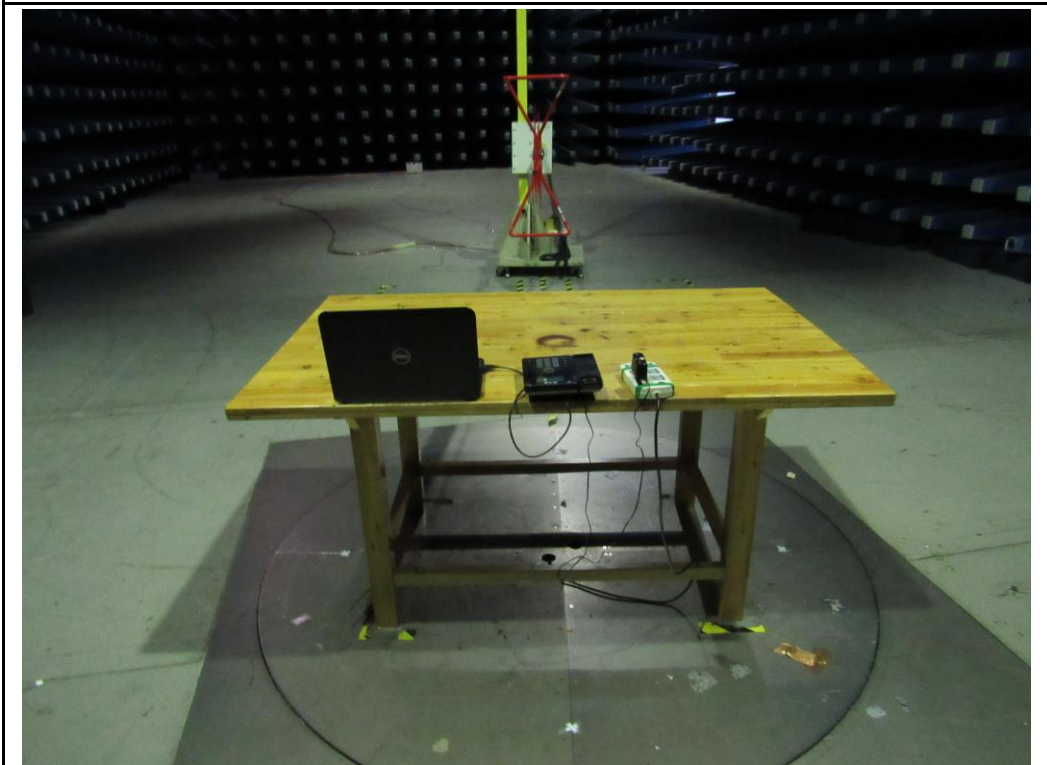
Radiated Spurious Emissions Test Setup Rear View Below 1GHz
