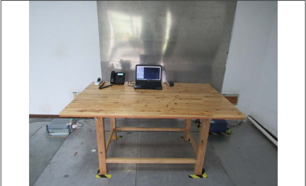
Conducted Emissions Setup Front View
