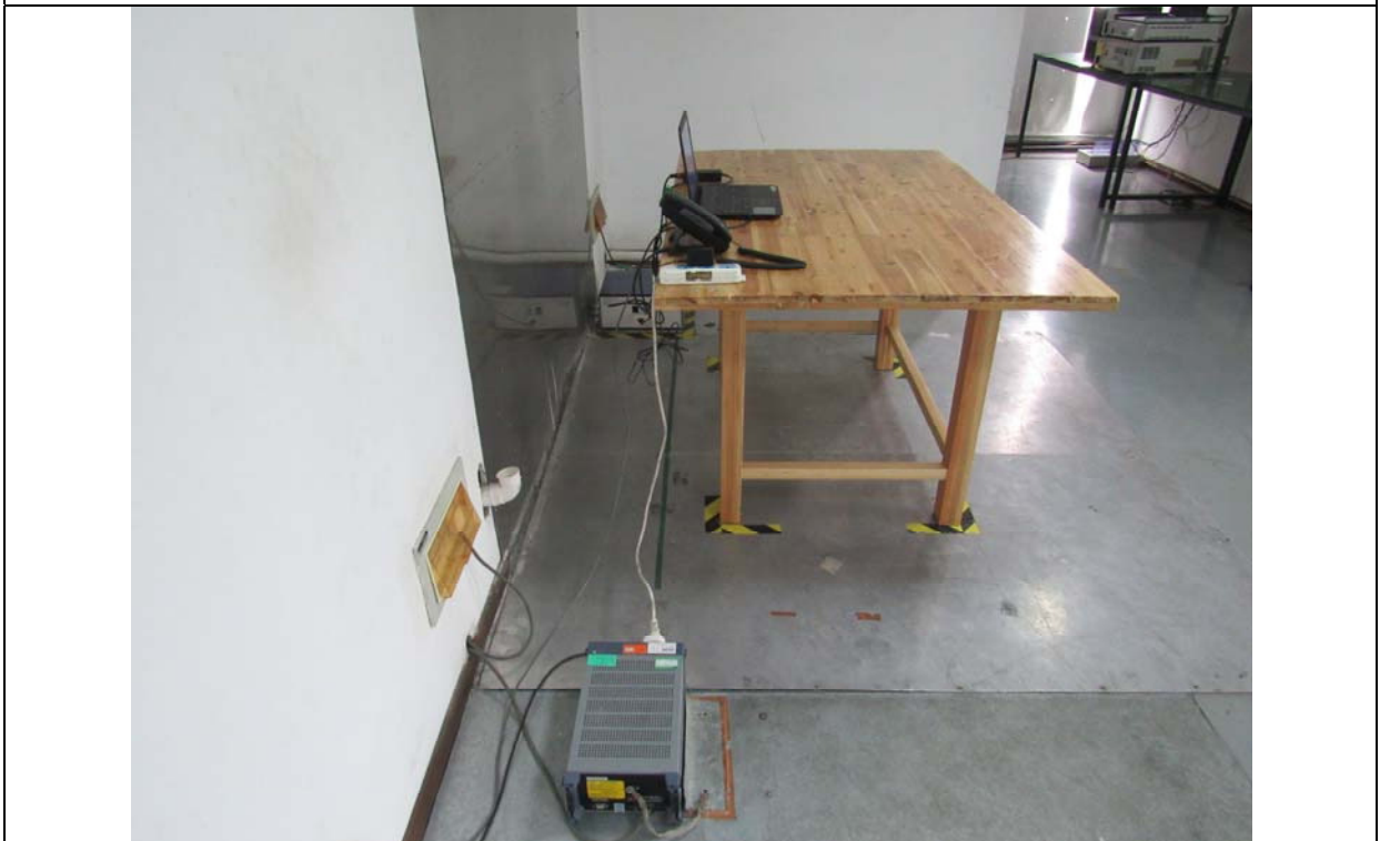
Conducted Emissions Setup Side View
