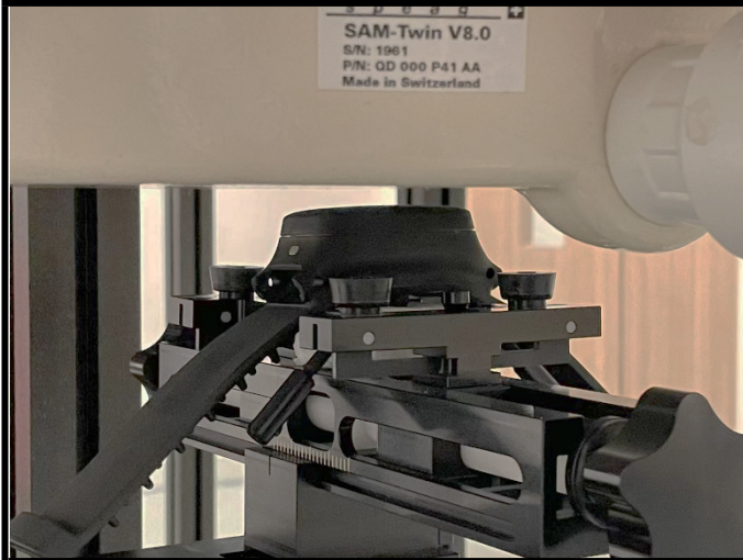
Front Face of EUT with 0.5 cm Gap
