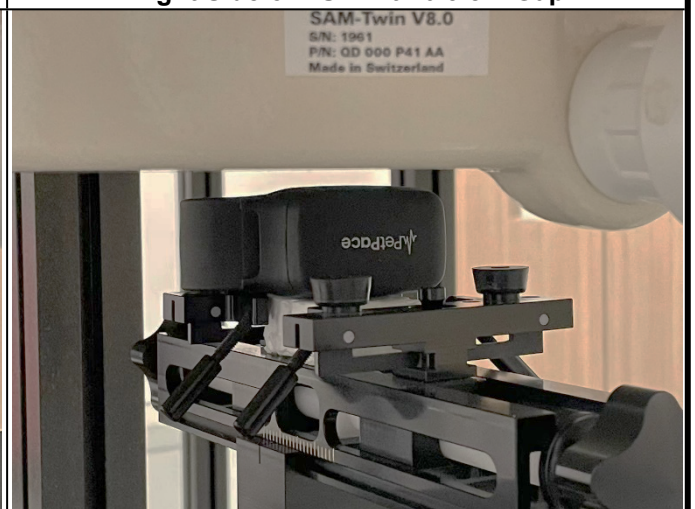
Bottom Side of EUT with 0.5 cm Gap
