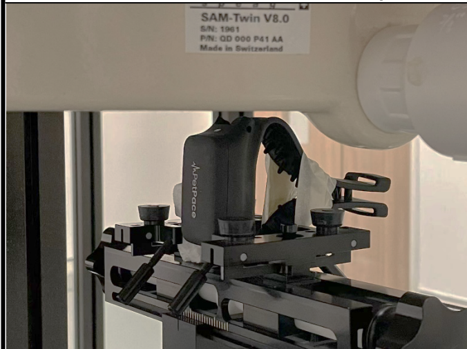
Left Side of EUT with 0.5 cm Gap
