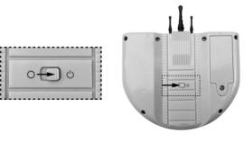
Remote controller will automatically pair with Droid. The pairing LED on the remote controller will start by flashing. Once paired, the LED will turn off signifying successful connection.
