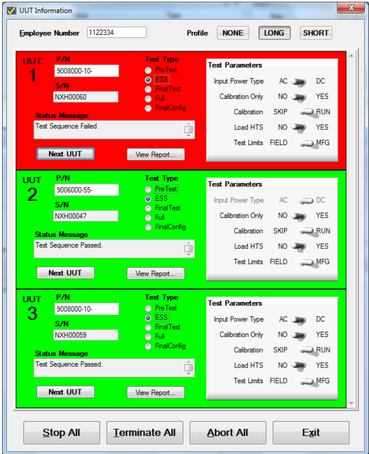
Figure 5-6: ESS/EIT UUT Information GUI (Tests Completed)
