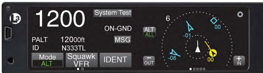
Figure 3-24: Example of Normal Operation
