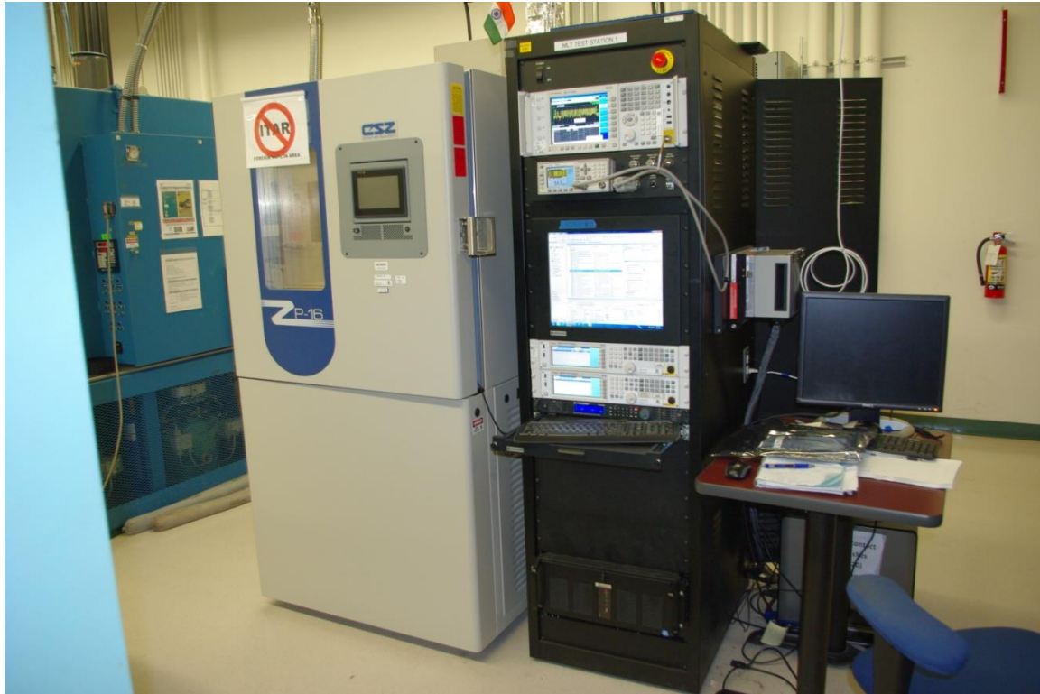
Figure 4-2: Test Equipment Setup and Temperature Chamber (Typical)
