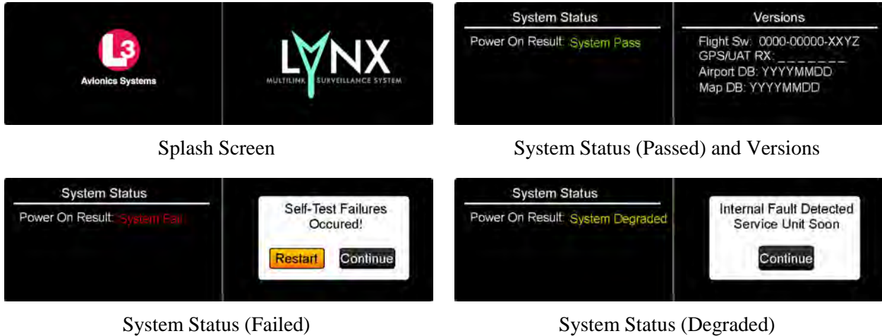
Figure 3-19: Examples of Start-up Screens
