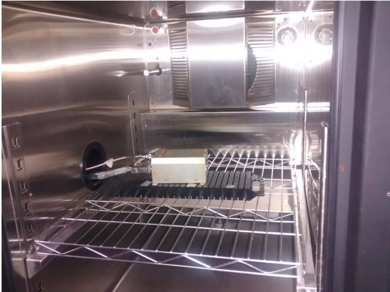
Figure 4-3: NGT-2500 inside the Temperature Chamber
