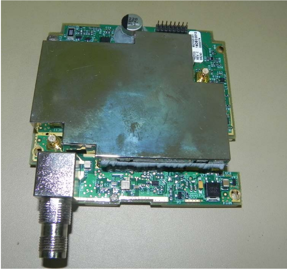
Figure 5-11: Power Amplifier CCA Top Side
