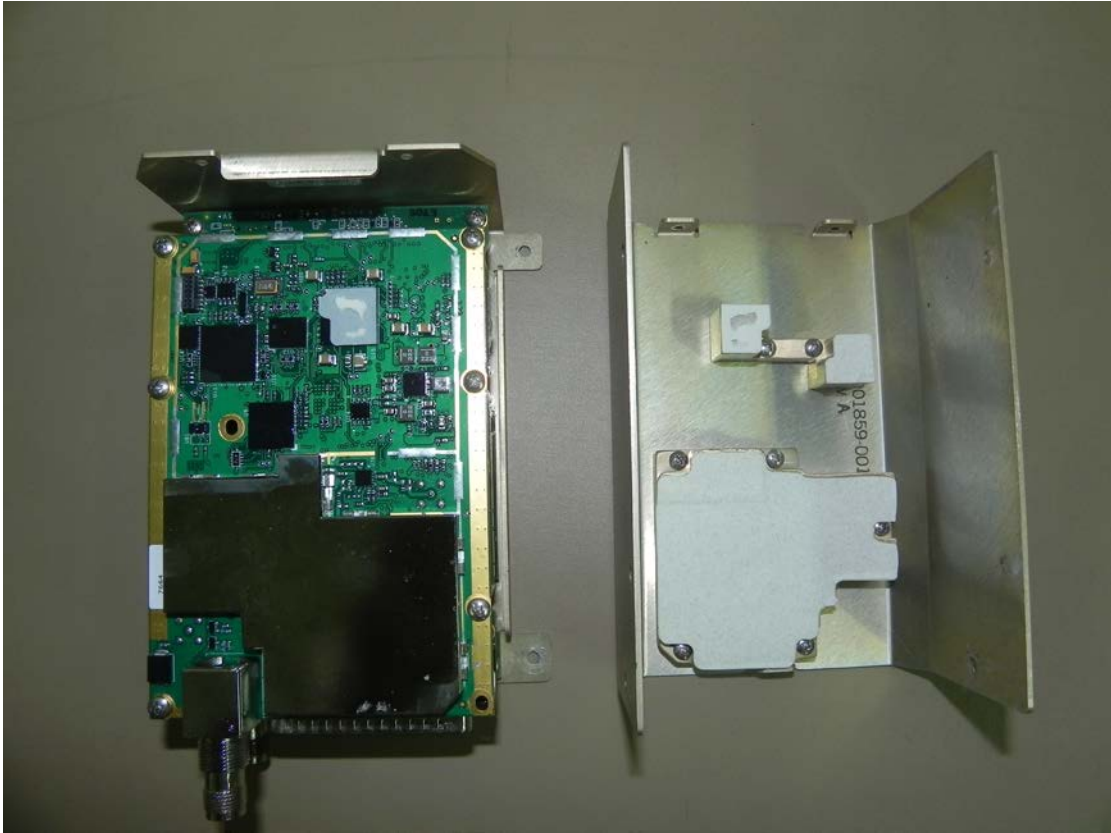
Figure 5-3: NGT-2500 Top View With Top Cover Removed
