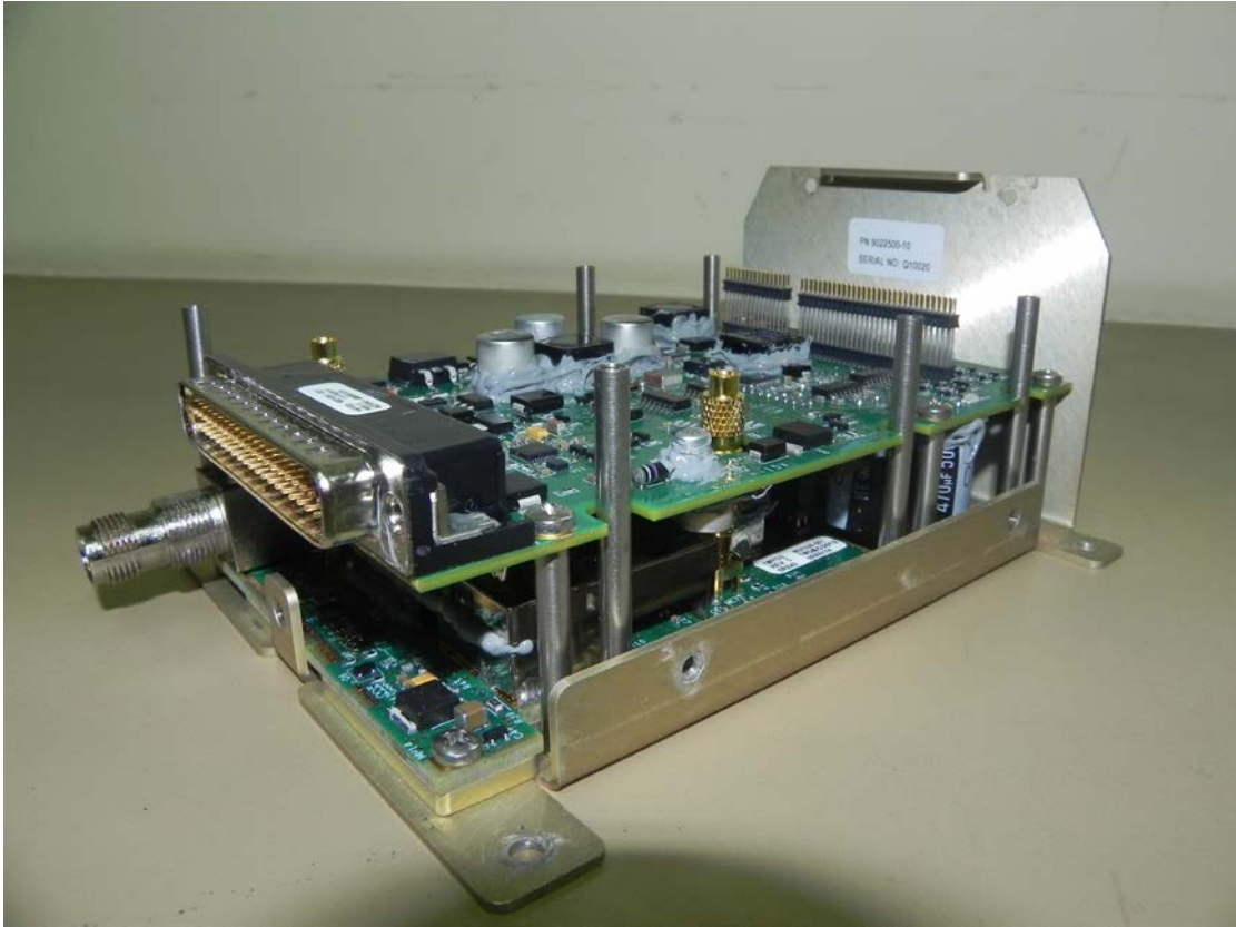
Figure 5-5: NGT-2500 with GPS-UAT CCA Removed
