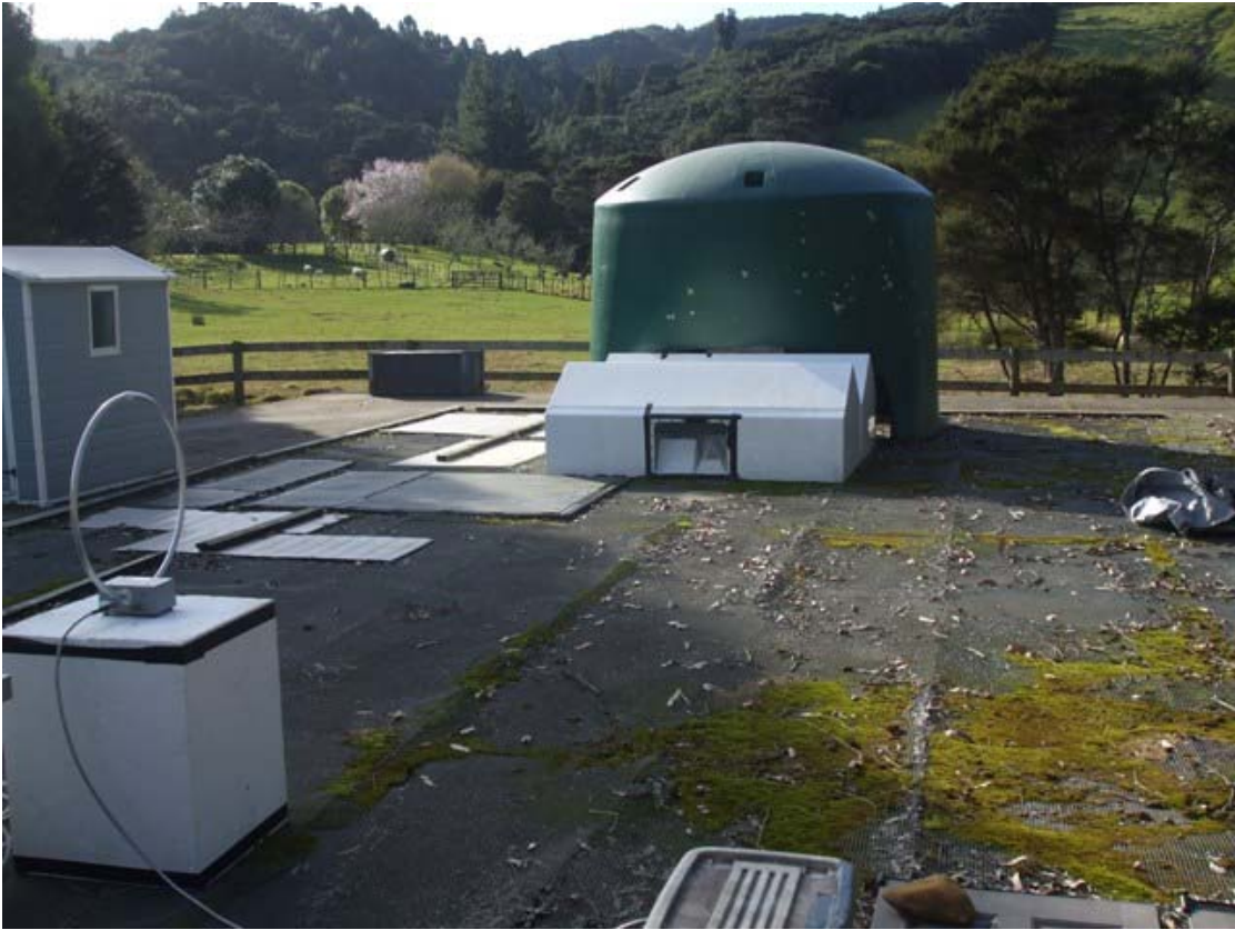
Loop Test Set Up. 100 kHz - 30.0 MHz
