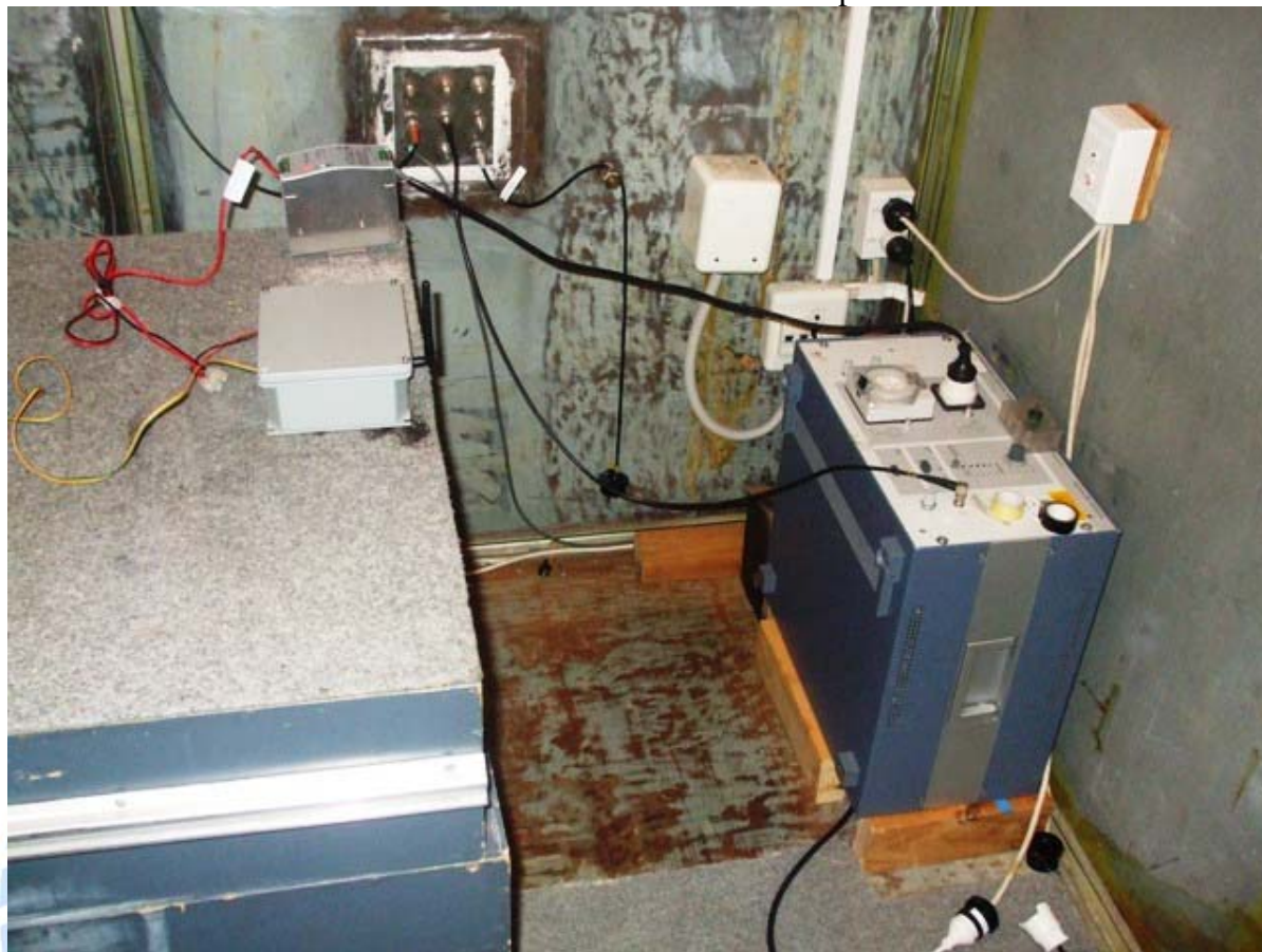
Conducted emissions test set up
