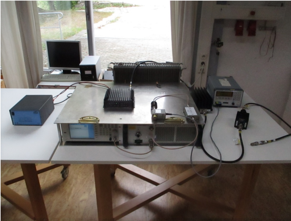
Photo A1-1: Conducted amplifier gain measurement
