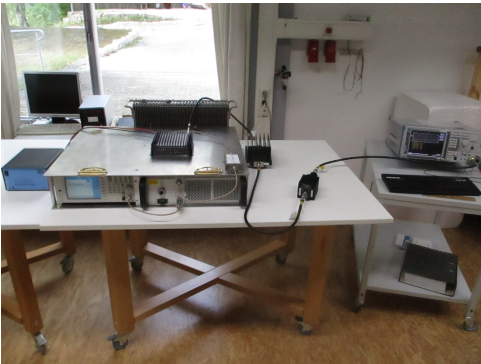
Photo A1-2: Conducted spurious emissions measurement
