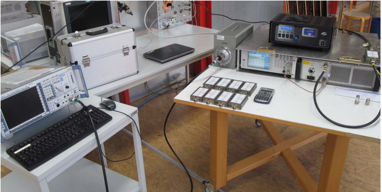
Photo A1-1: Conducted amplifier gain and spurious emissions measurement
