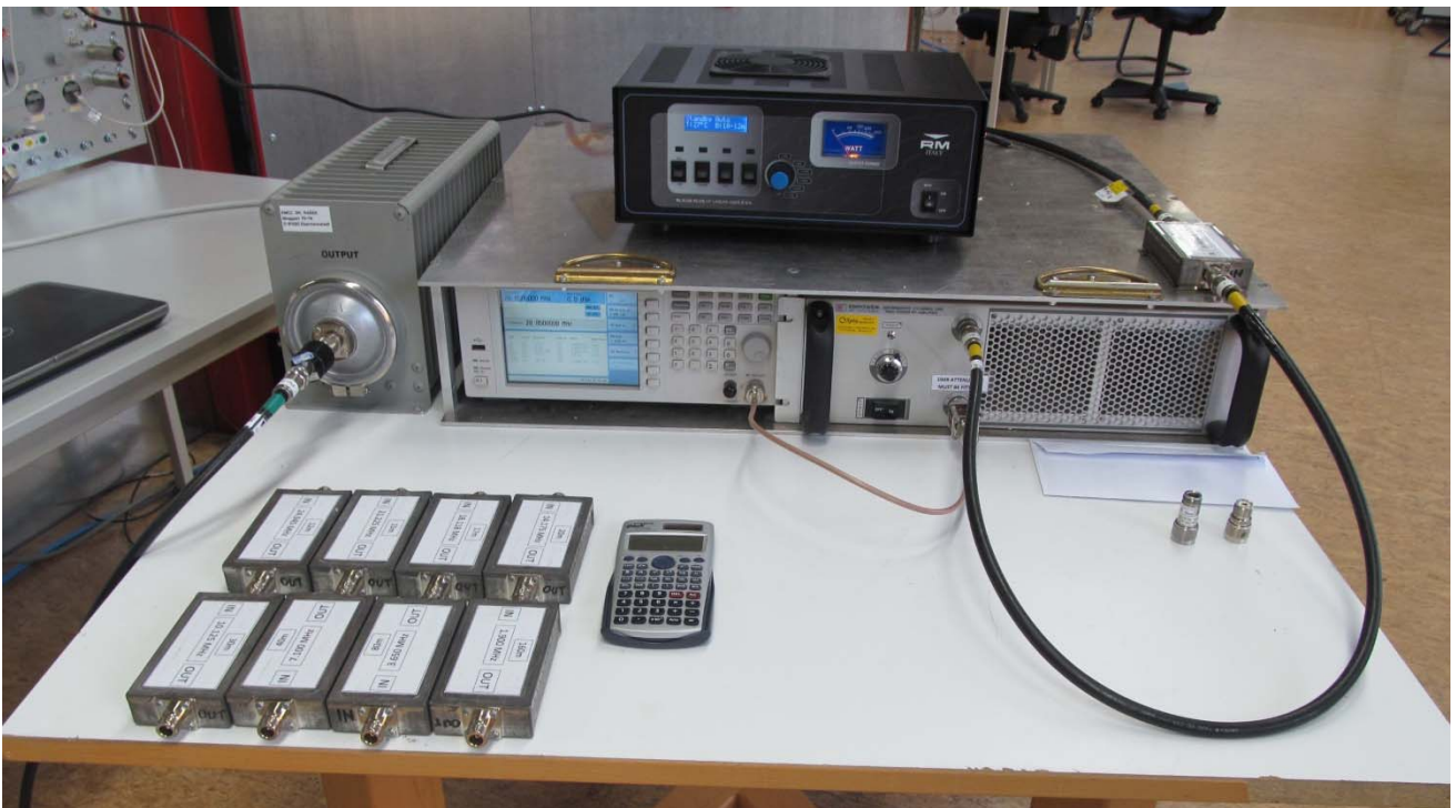
Photo A1-2: Conducted amplifier gain and spurious emissions measurement (detail view)
