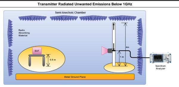
Magnetic field tests shall be performed in the frequency range of 9 kHz to 30 MHz using a calibrated loop antenna. Electric field tests shall be performed in the frequency range of 30 MHz to 1000 MHz using a calibrated bi-log antenna.
