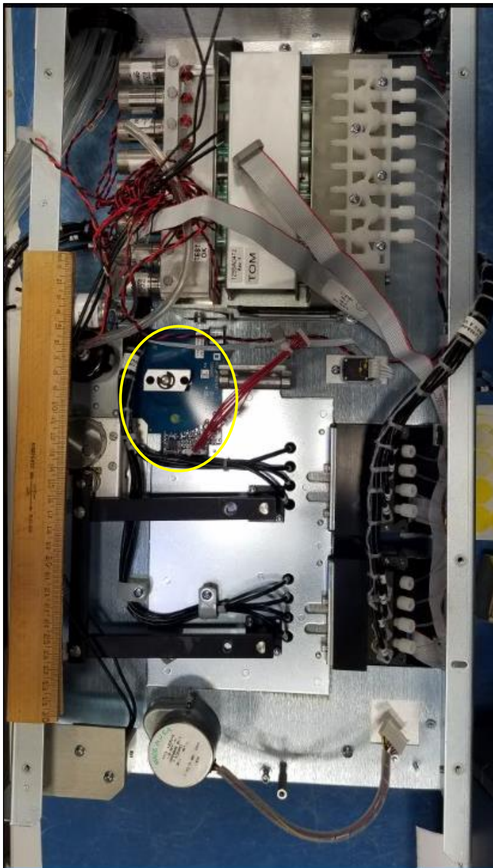
Figure 4: Chemcassette® Analyzer Parts Removed to Show Installation of RFID Circuit Board
