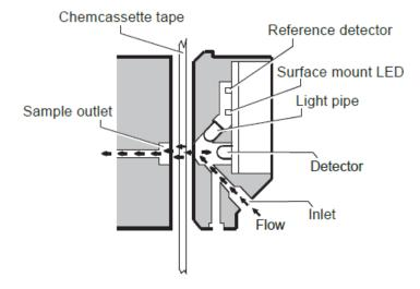
The microprocessor in the Chemcassette analyzer module interprets the stain. It then calculates and stores a precise concentration level in the module's memory. Gas concentrations are reported in parts-per-million (ppm), parts-per-billion (ppb) or milligrams-per-cubic-meter (mg/m<sup>3</sup>).
