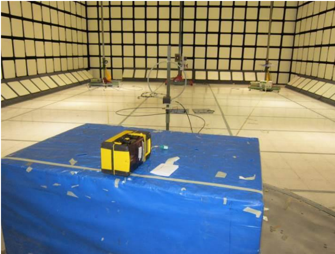
Figure 10 Test Setup for Radiated Emissions
