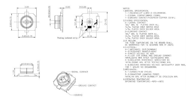
Figure 7. 1<sup>st</sup> IPEX Connector
