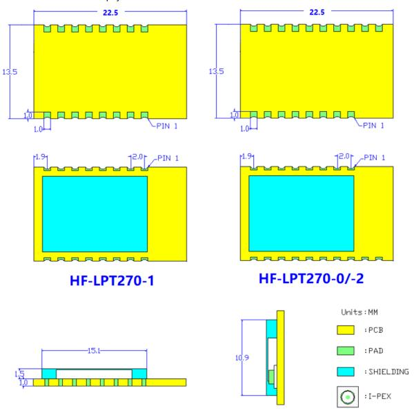
Figure 5. HF-LPT270 Mechanical Dimension
