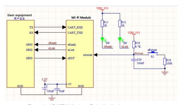
Figure 11. HF-LPT270 Hardware Typical Application
