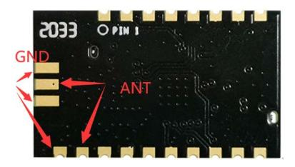
Figure 4. HF-LPT270-2 Antenna PAD Out
