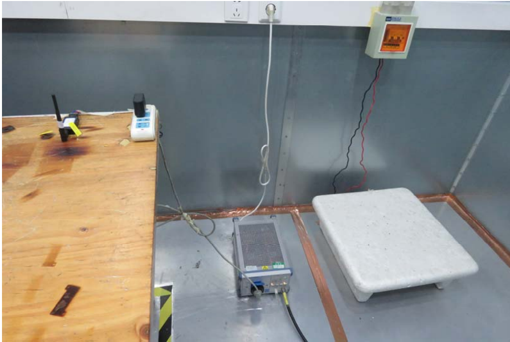
Picture 2: Conducted Emissions Test Setup
