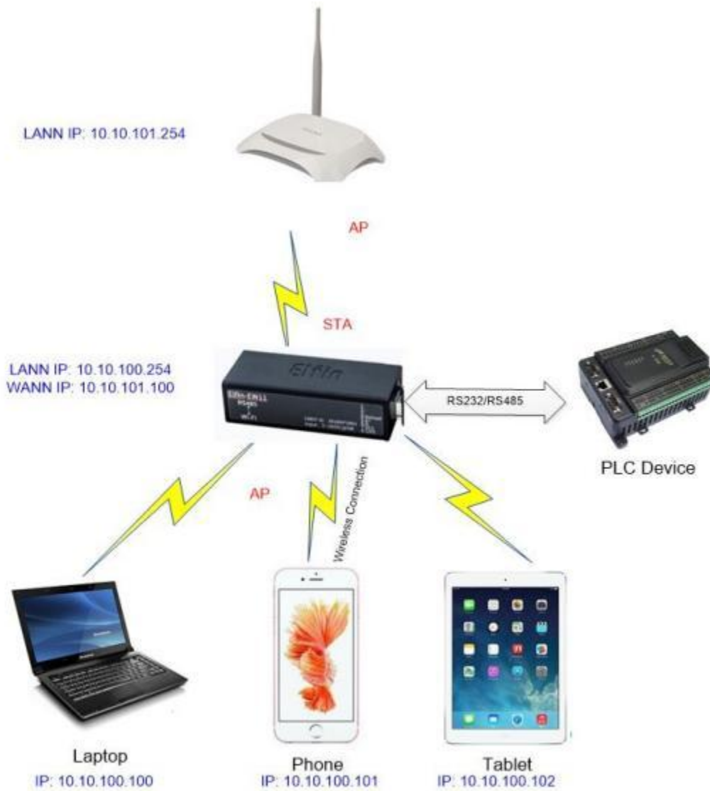
Figure 30. AP+STA Wireless Network
