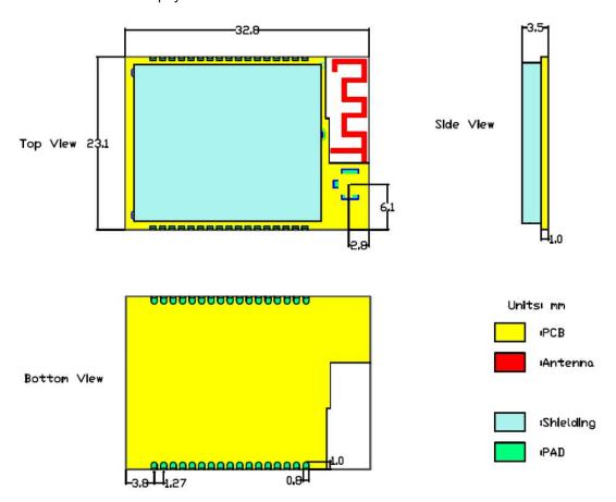
Figure 4. HF-LPB170 Mechanical Dimension
