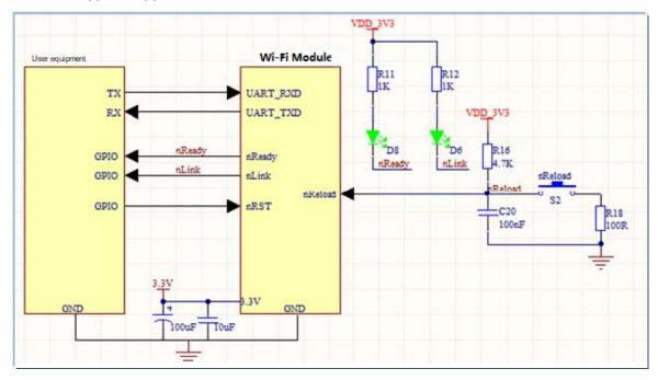
Figure 7. HF-LPB170 Hardware Typical Application
