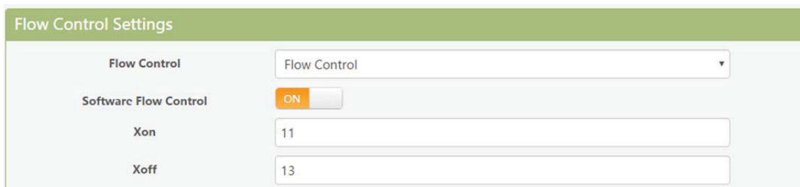
Figure 45. UART Flow Control
