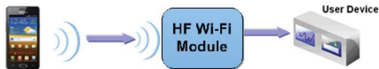
Figure 31. Wireless Control Application
