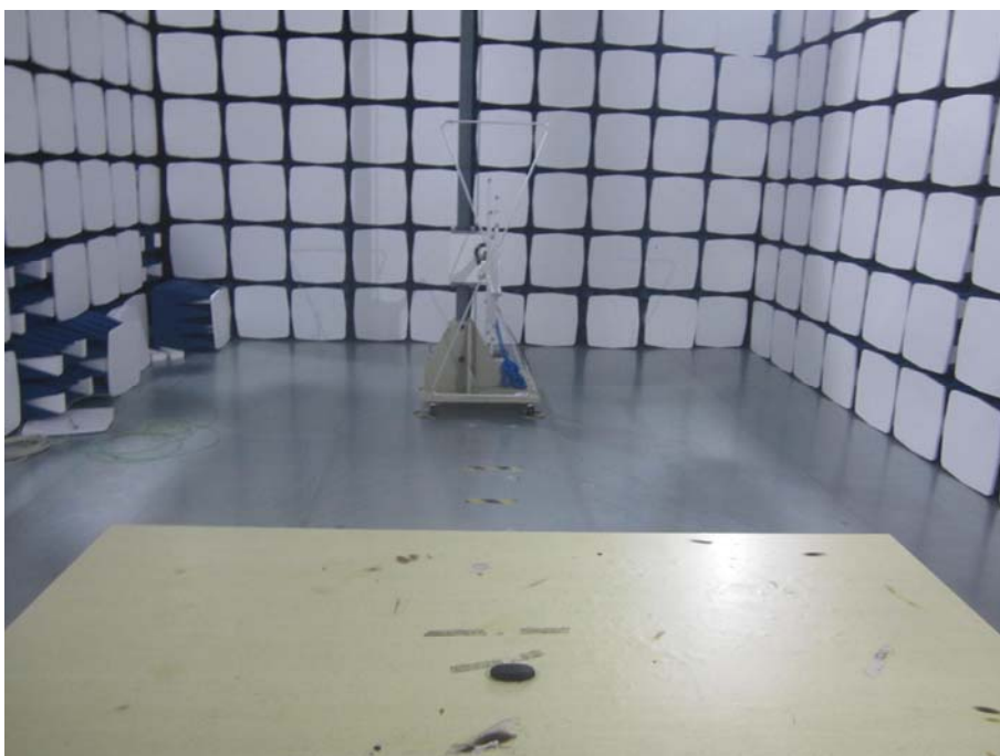
Radiation Emission Test Setup (30MHz to 1GHz)
