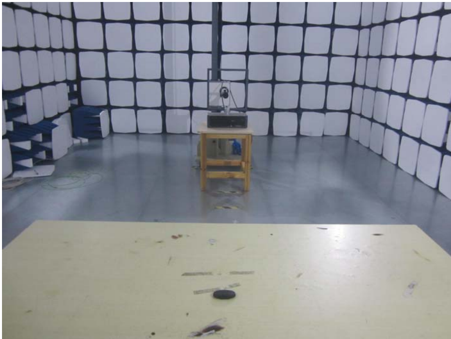
Radiation Emission Test Setup (Below 30MHz)
