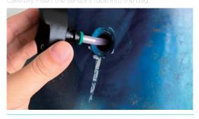
Your new sensor will arrive sealed with shrink wrap. The recommendation is to leave the shrink wrap on the sensor to protect it from water intrusion when inserting the sensor for the first time.
