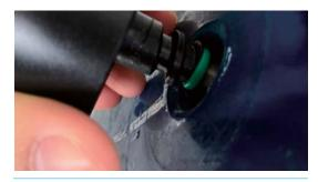
The sensor needs to be tight enough that no air is leaking around the threads, but caution should be used, as over-tightening the sensor could damage it.
