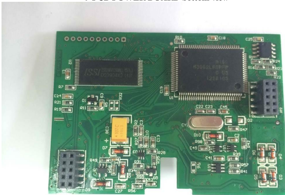
9 PCB POWER BOARD bottom view
