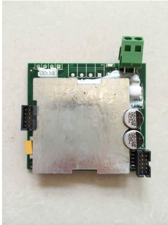
7 PCB POWER BOARD top view with shielding
