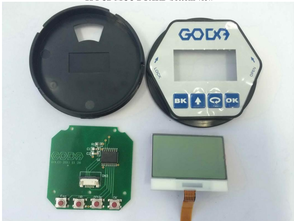
12 PCB DISPLAY BOARD top view
