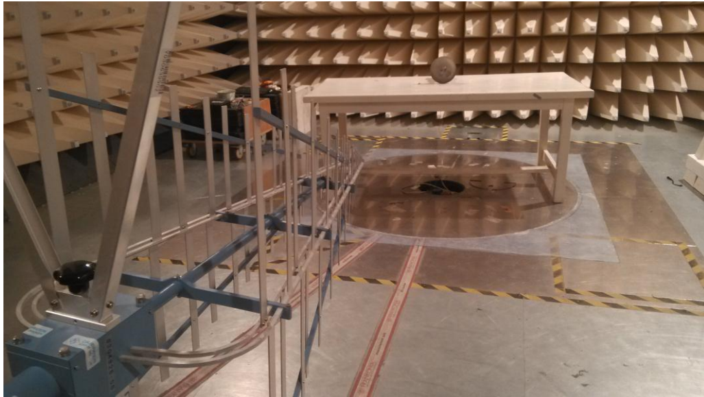
Photograph 2: Set-up for Spurious Emissions, above 1GHz
