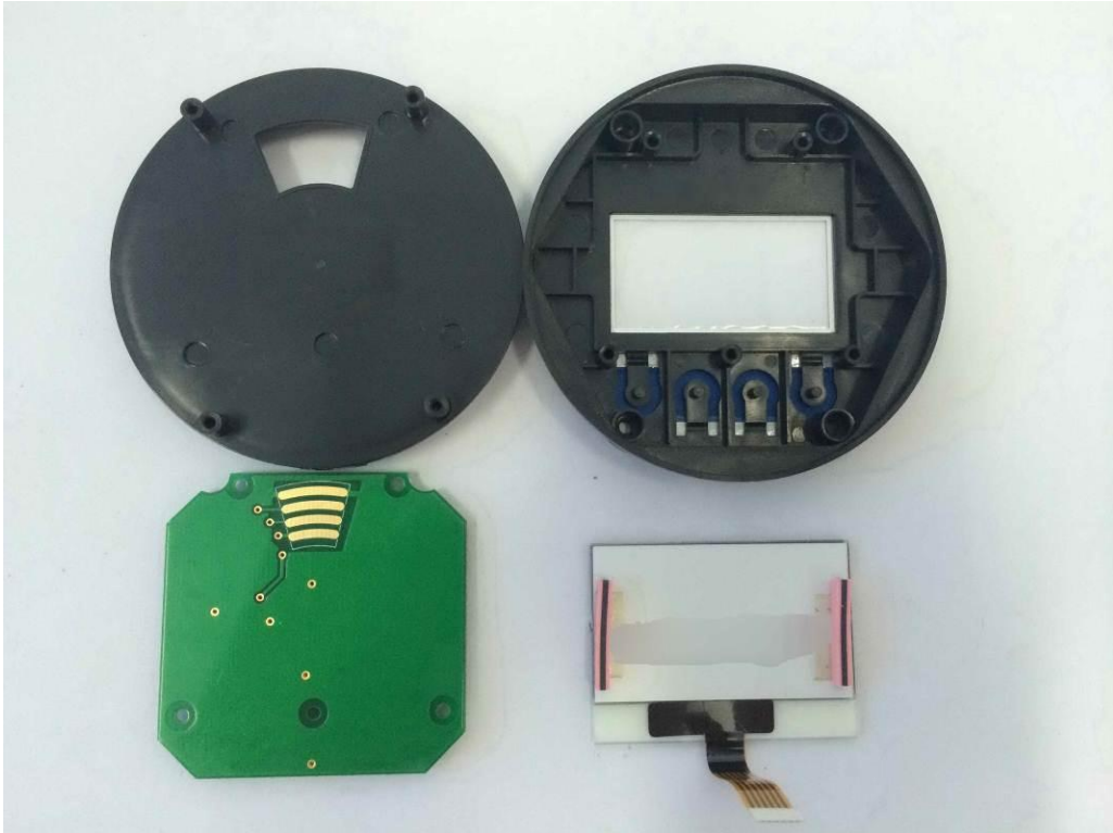
13 PCB DISPLAY BOARD bottom view
