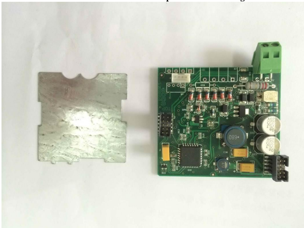
8 PCB POWER BOARD top view without shielding
