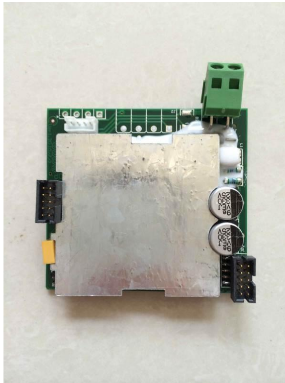
7 PCB POWER BOARD top view with shielding
