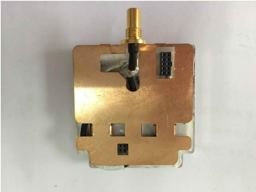
15 PCB HF BOARD bottom view with shielding
