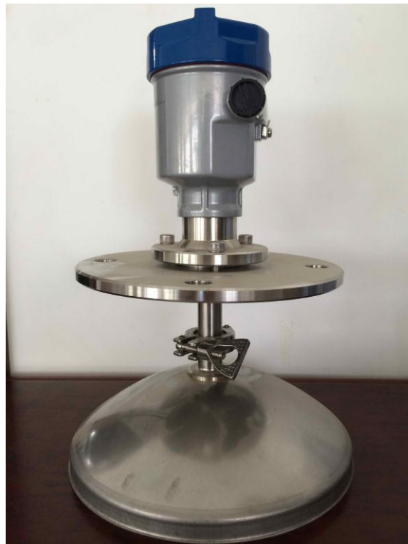
6 Side view of GDRD58 with PARABOLIC ANTENNA
