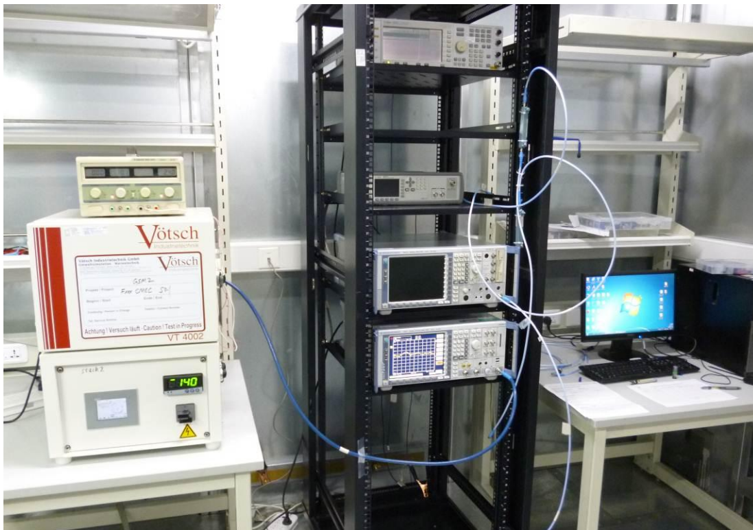
Photograph 3: Set-up for Fundamental emission bandwidth and Frequency stability test
