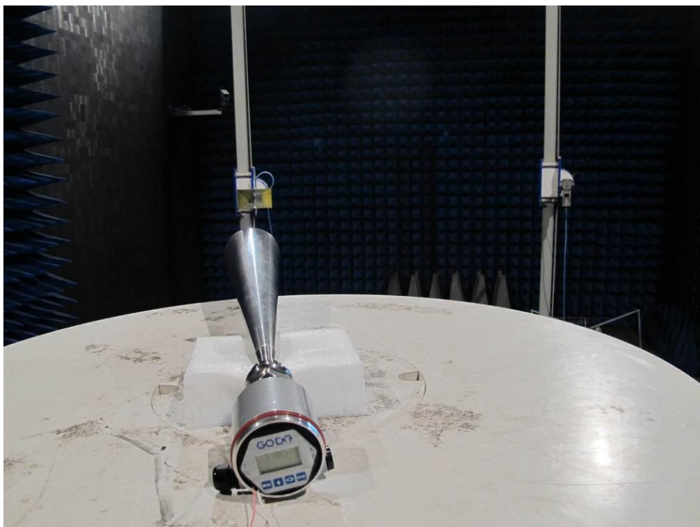
Photograph 2: Set-up for Spurious Emissions, above 1GHz
