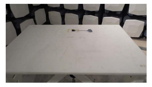
13.2 Radiated Emission below 1 GHz Rear View at 3 Meters
