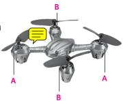
To replace a damaged blade, use a screwdriver to remove the old blade. Insert a new matching blade onto the blade axle, then screw securely.
