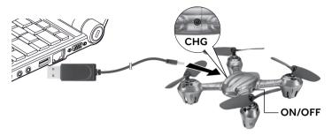
Connect the included USB charging cable to the drone's CHG jack and a USB power source (such as a laptop). The LED inside the USB connector lights red during charging, and turns off when charging is complete.
