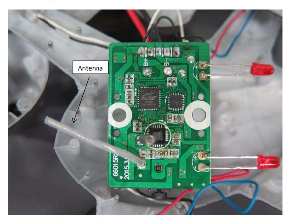
Antenna of this product is unique antenna and unchangeable; fulfill the requirement of this section
