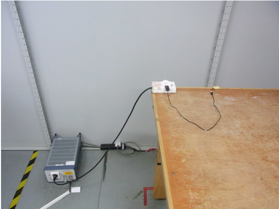
Conducted emission (Front view)
