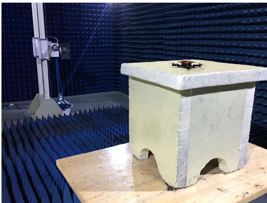
Photograph of set-up for Radiated Emission above 1GHz
