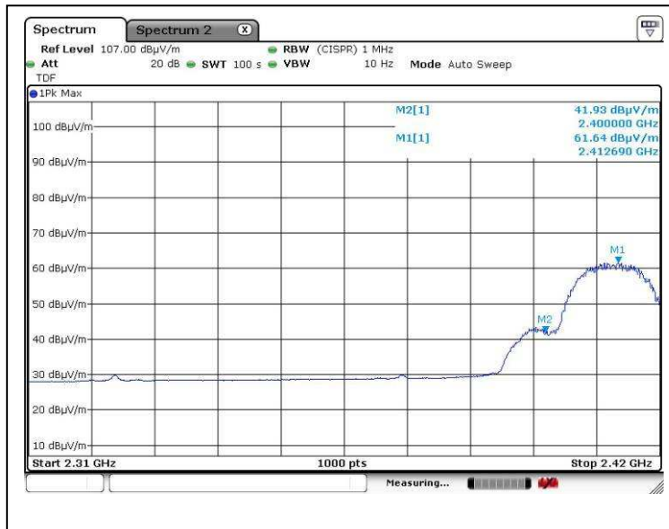
802.11b lower edge (Average measurement)
