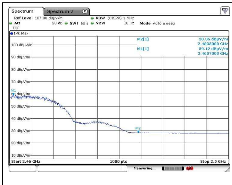
802.11b higher edge (Average measurement)
