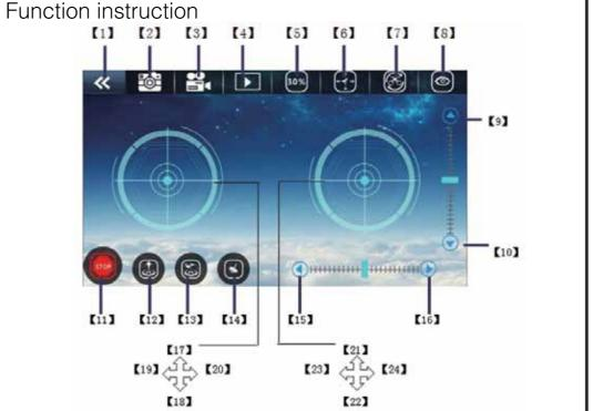
1] Return [2] Take photo [3] Video record [4] Photo&video playback [5] speed [6] headless mode [7] Flip fly [8] Show/Hide control intertace [9] Fine tune forward [10] Fine tune backward [11] Stop [12] one button take off and landing [13] one button fly back [14] Motion control [15] Fine tune left [16] Fine tune right [17] Ascend [18] Descend [19] Turn left [20] Turn right [21] Forward [22] Backward [23] Slide left [24] Slide right
