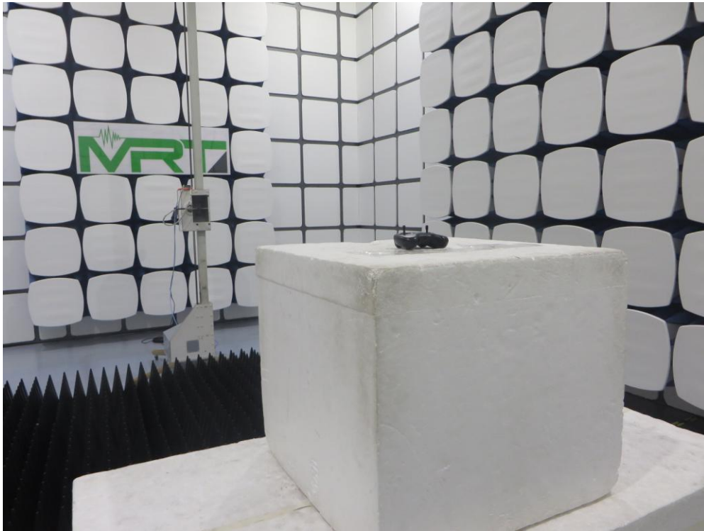
Description: Radiated Emission Test Setup (18GHz ~ 25GHz)
