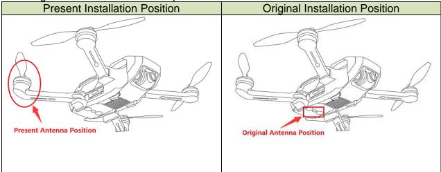
The antenna is the same except for the installation position.
