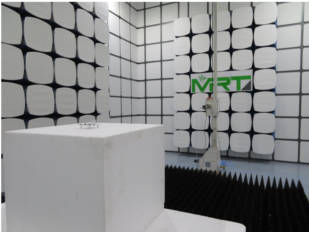
Description: Radiated Emission Test Setup (18GHz ~ 40GHz)
