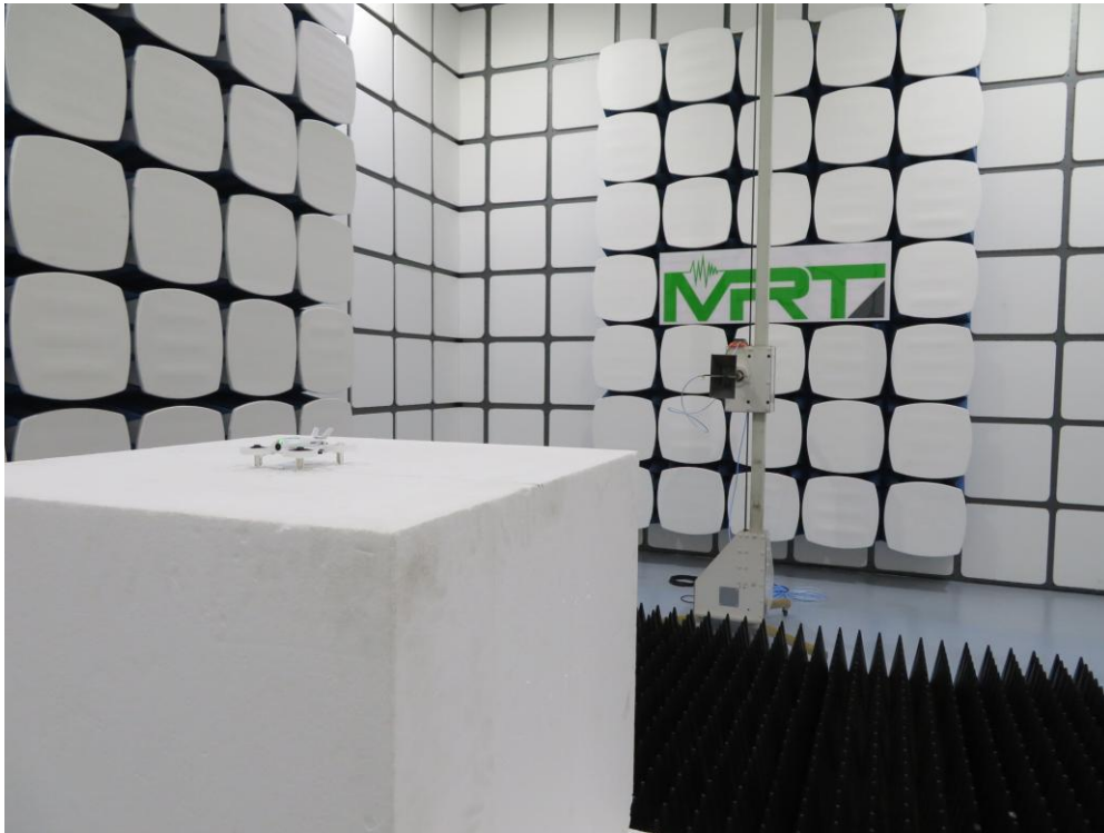
Description: Radiated Emission Test Setup (18GHz ~ 40GHz)
