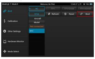
• The receiver/model should now be bound to the ST24. Or, if the receiver/model was not bound successfully repeat the steps outlined above to complete the binding process.
