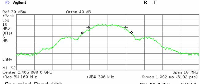
Occupied Bandwidth 2.6898 MHz Occ BW % Pwr 99.00 % -6.00 dB x dB
