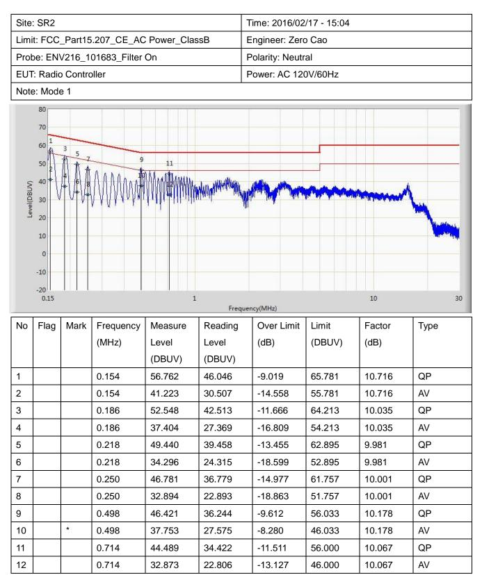
Factor (dB) = Cable Loss (dB) + LISN Factor (dB)
