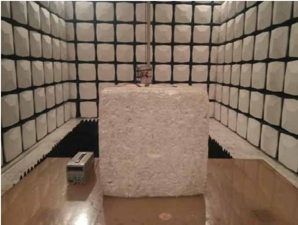
Description: Radiated Emission Test Setup for 1~18GHz
