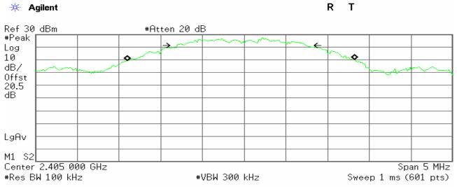
Occupied Bandwidth 2.7236 MHz Occ BW % Pwr 99.00 % x dB -6.00 dB
