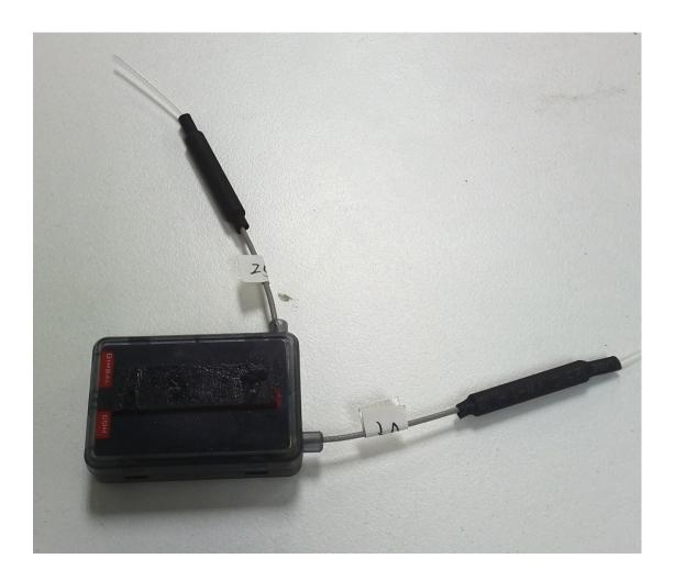
Plug the cable from FCO(flight control for HX4) into SR12E socket, and power on HX4. Lean HX4 nose forward twice times, the BLUE LED of SR12E will flash slowly, indicating the receiver ready for binding. When the binding between SR12E and ST24 completes (see the following instructions of **Binding HX4 and ST24**), the BLUE LED will be off. Turn on ST24, press FPV and press 'Take off'.
